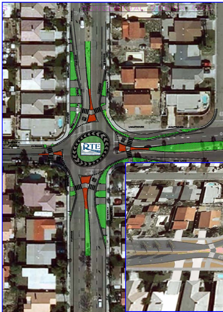
Example of small SLR with an elliptical shape designed to fit within ROW constraints where a circular roundabout would not function well for proper speed control or large truck movements (N and E legs designated local truck route). (Note: Animated image below is rotated)
